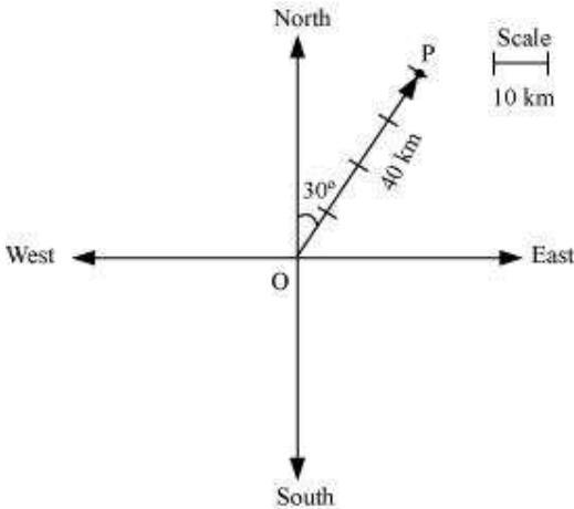
Here, vector  $\overline{OP}$  represents the displacement of 40 km,  $30^\circ$  East of North.
